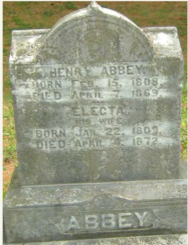
Figure 9. Irreversible damage caused by a wire brush. Photo by Andrew L.—Find A Grave.
