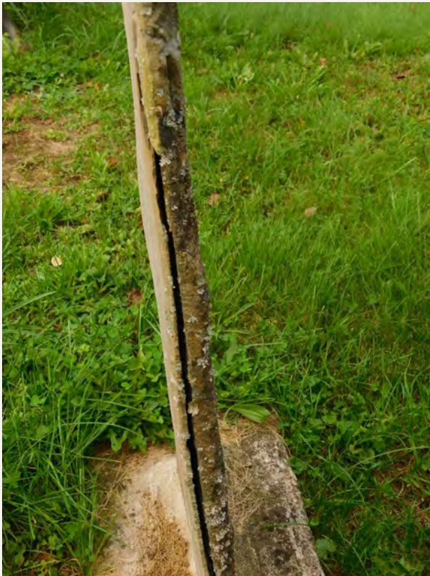
Figure 1. An example of a gravestone splitting apart due to delamination.
